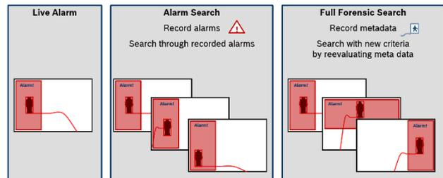
The second part of the configuration evaluates the metadata and includes tasks like line crossing, object in field and more. This second part can be fully evaluated and optimized using forensic search. To do so, record video including the events to be detected. Then use a forensic search capable viewing client like BVC. Define or adapt your alarm tasks, and evaluate whether all events are detected correctly and how many false alerts are still left.
