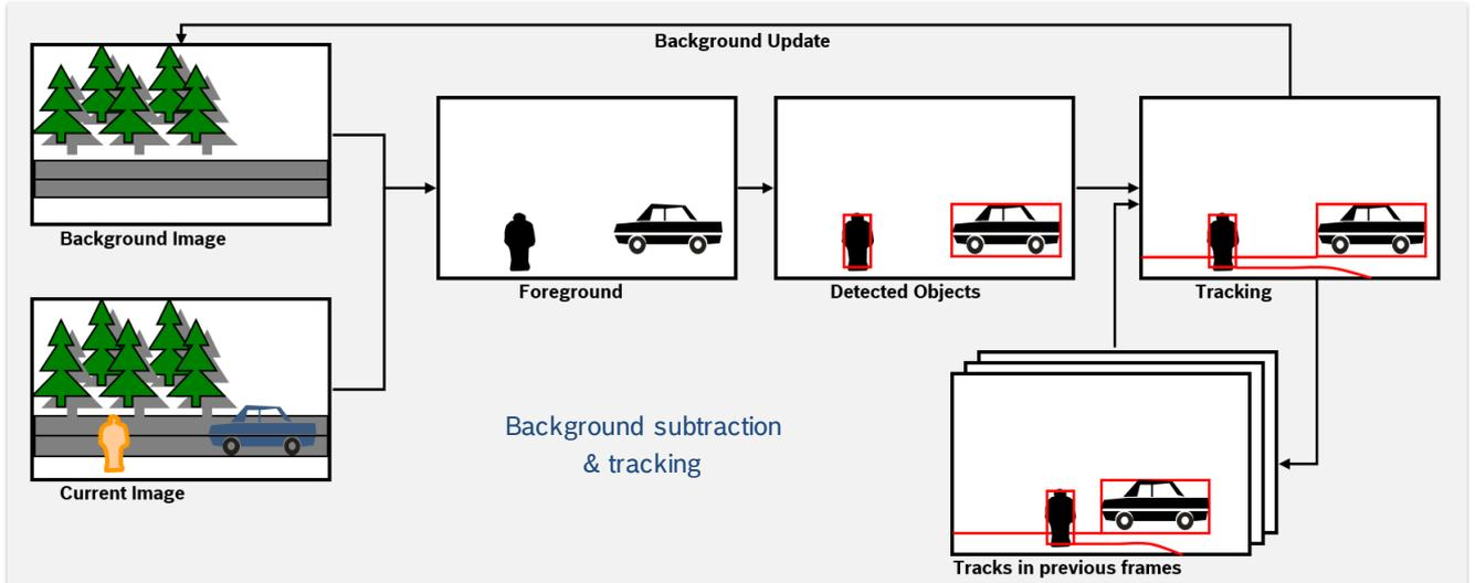
Now for all three technologies, if the wind moves a branch, then there is a distinct change to the position of the branch a second ago and the branch is detected as a potential change / motion / moving object. By combining the different technologies, tracking the objects over time and evaluating the consistency of motion, robustness can be achieved even to these kind of moving objects the user is typically not interested in.
