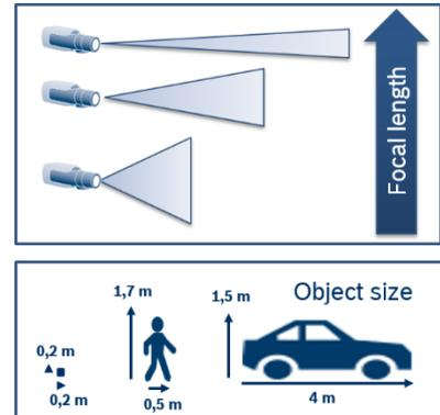
Distance resolution is best near the camera, and degrades heavily into the distance where a single pixel in the internal resolution often covers several meters of ground. Here an example for Essential Video Analytics:
