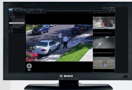
An alarm coming from a device or detector connected to the BIS server can trigger video verification of the alarm on XProtect client. The operator can then zoom in for details and further investigate the scene with more cameras before responding to the alarm.
